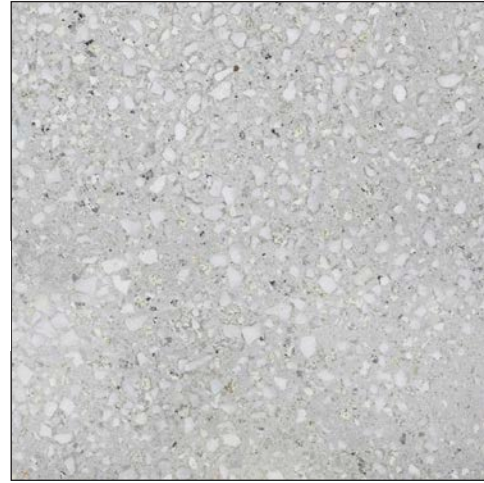
Concrete Paving with Exposed Aggregate
