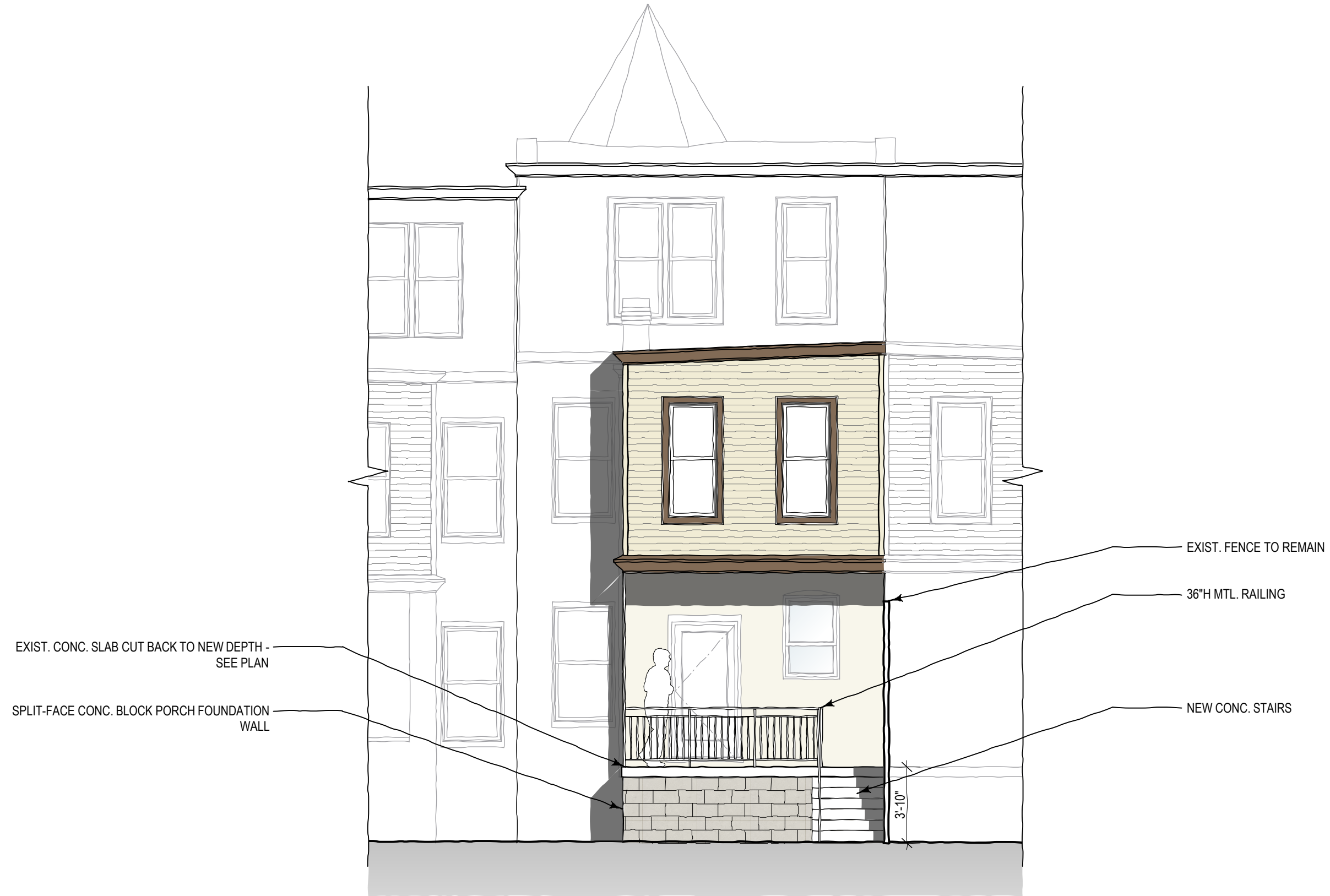
1 PROPOSED REAR ELEVATION Scale: 3/16" = 1'-0"
