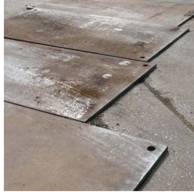
Reclaimed steel plates
